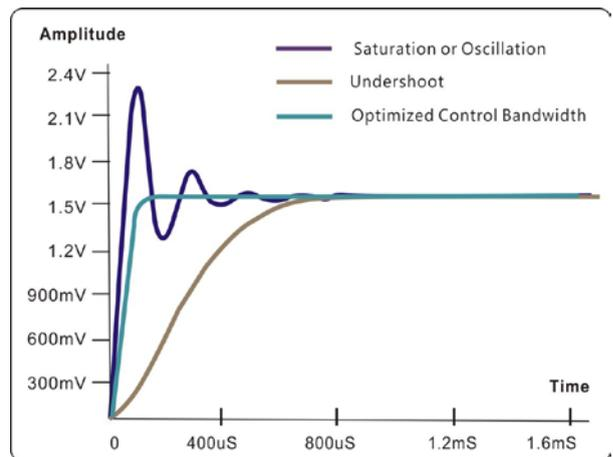
Figure-3 1.5V Step Response with 0.1 uF Capacitor as capacitive Load
