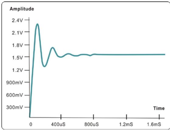
Figure-2 1.5V Step Response with 0.1 uF Capacitor as capacitive Load
